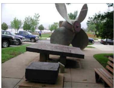
Shown in the photograph to the left are 3 artifacts removed from USS SOUTH DAKOTA (BB-57.) In the foreground is a 16" steel belt armor plate section which once ringed the waterline hull of SOUTH DAKOTA. The middle plate is a partial top section of SOUTH DAKOTA's Turret #1, and next is a 36,000 pound manganese bronze propeller, manufactured for SOUTH DAKOTA at the Philadelphia Navy Yard. These screws produced 179 rpm and were capable of 28 knots for the 35,000 ton ship.
