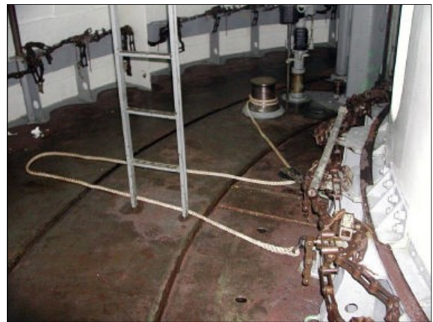
Projectile flat - found three decks below in each of the three Main battery (16") turrets. Stored projectiles, chained and secured along the turret sides, would be manually maneuvered over to the projectile hoist seen at top right.
