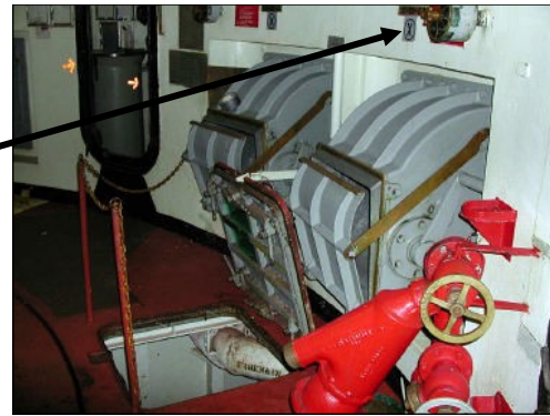
Scuttle loader control above each scuttle station. Found on the bulkheads of the lower powder handling rooms of the three Main battery (16") turrets - 5 decks below.
