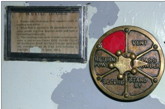
Scuttle loader control above each scuttle station. Found on the bulkheads of the lower powder handling rooms of the three Main battery (16") turrets - 5 decks below.
