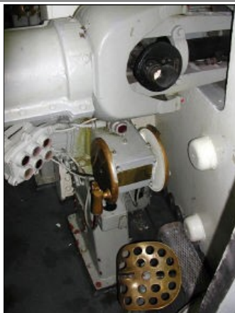
Powder magazine tray used to roll the 110 pound powder bags into the Scuttle loaders.
