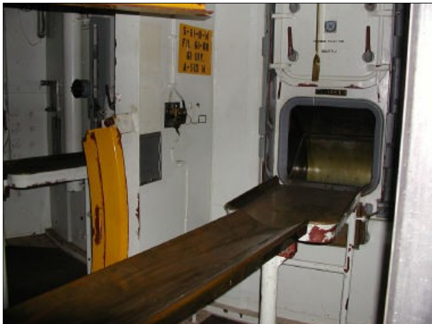
Powder magazine tray used to roll the 110 pound powder bags into the Scuttle loaders.
