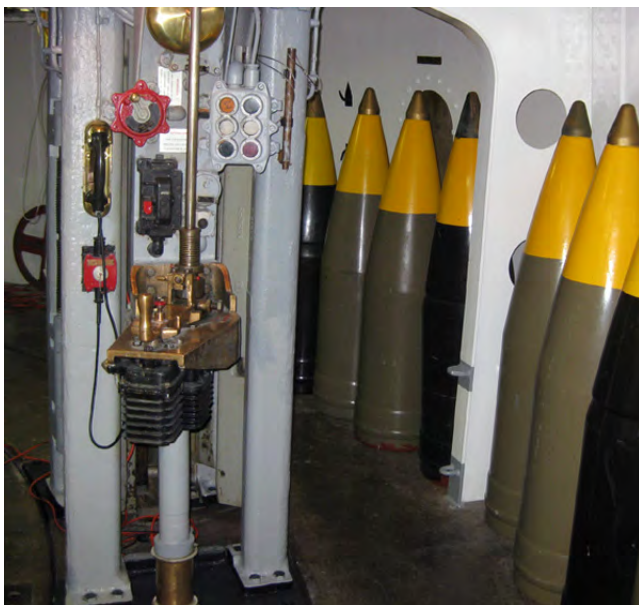
1. Load a shell into a hoist and send it up to the gun.
