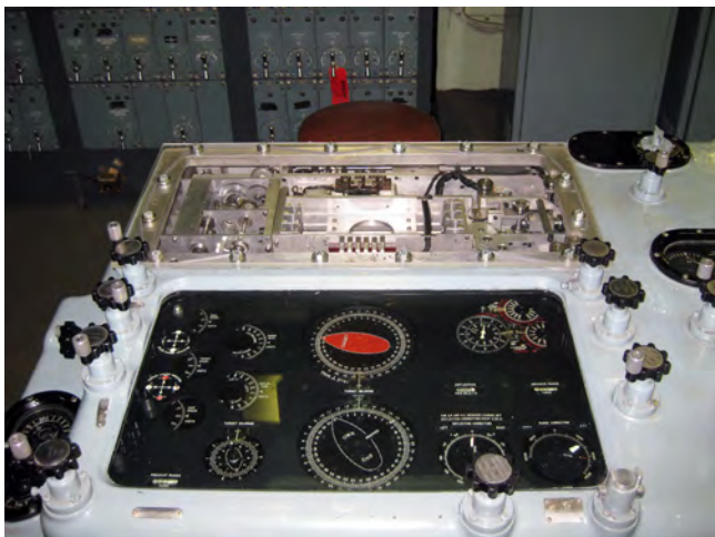
Mark 8 Range Keeper in Forward Main Battery Plot
