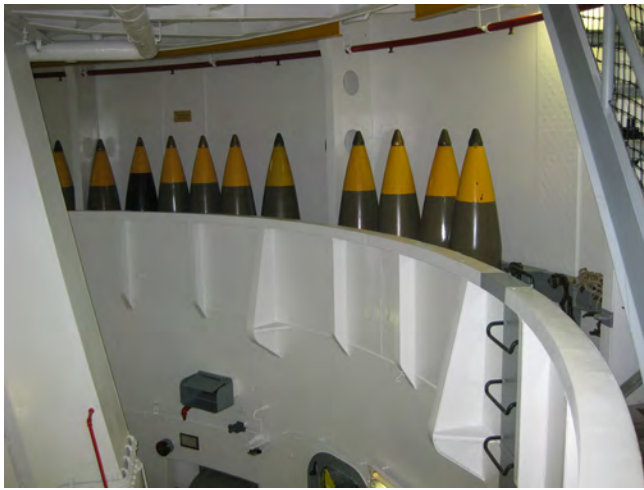
Open 3 rd Shell Deck of Turret 2
