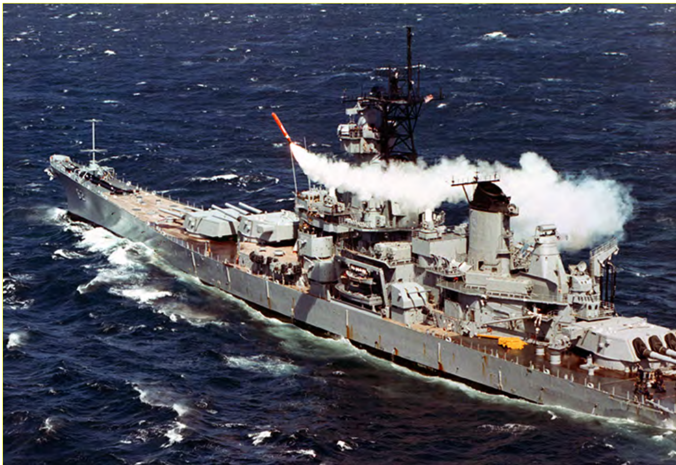
Aerial port quarter view of USS New Jersey during the launch of a Tomahawk missile from one of her eight Armored Box Launchers, May 10, 1983. At the time the battleship was off the coast of Southern California, and the missile traveled approximately 500 miles to its target at the Tonopah Test Range in Nevada. Official U.S. Navy photo # DN-SC-83-08071
